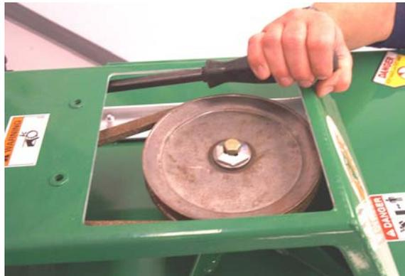
Adjusting Blade Drive Belt Tension
